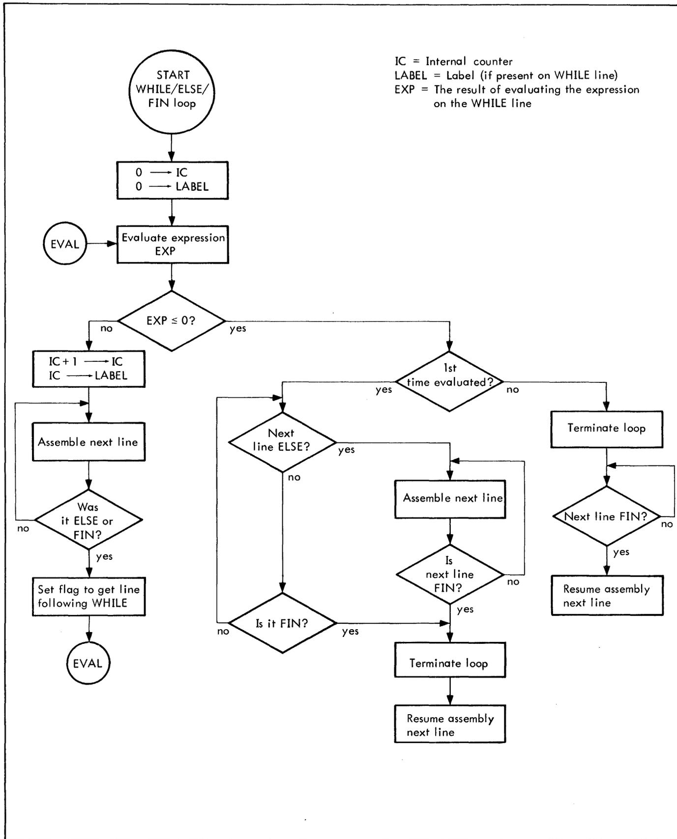
Figure 2. Flowchart of WHILE/ELSE/FIN Loop
