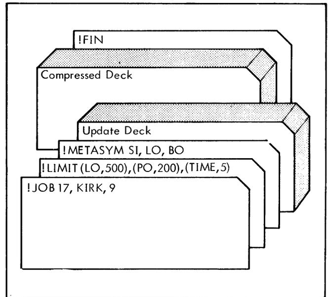
Figure 14. Sample Run Deck – Single Assembly with Update
